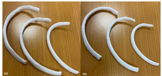
Figure 7. 3D printed rib models of rib 4. The original model is placed in the middle, the statistical model on the right side and the mirrored on the left side. (a) Patient 5 (b) Patient 1.
