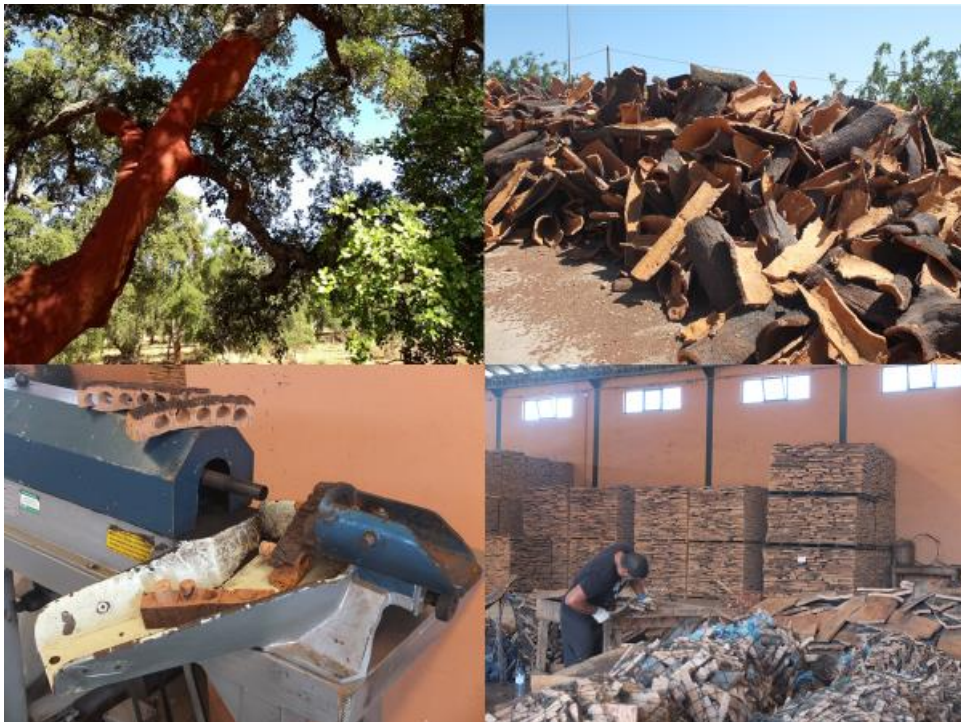
Figure 1. Clockwise from top left: cork tree stripped of bark, cork bark sections, stabilized cork planks being trimmed, cork punching machine (Source, Authors' own photographs)
