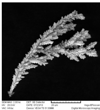
Figure 1. SEM photomicrographs of copper powder particles obtained in constant current deposition.
