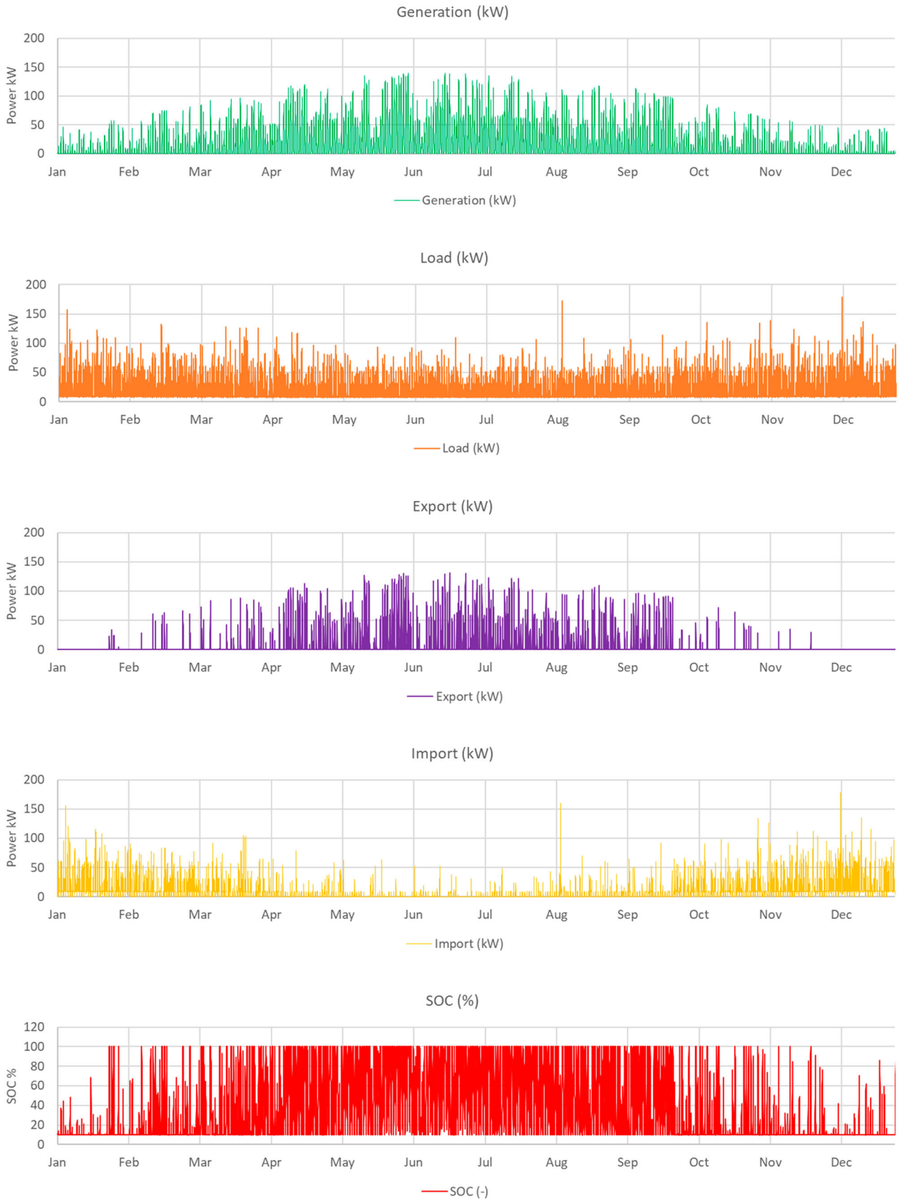
Figure 13. Example of time series output from the simulation, for the case with 50 vehicles and 100 kWh battery.
