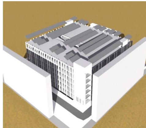
Figure 9. Duke St car park (Image: Google street view) and rendered image of the ESP-r Duke St Car Park model with roof-mounted PV arrays and shading from surrounding buildings.
