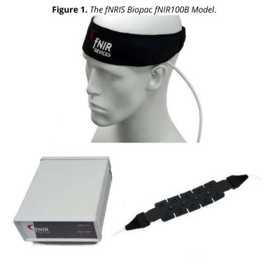
*Note.* This figure shows the hardware utilised to collect the level of HbO on the PFC of the subject. The box was connected to a computer loaded with Cognitive Optical Brain Imaging studio (COBI) software. Photo Courtesy of ©BIOPAC Systems, Inc.
