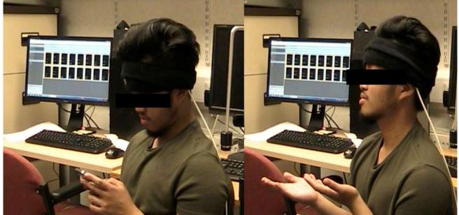
Figure 2. Flexible Sensor Band Fit on Subject's Forehead.
