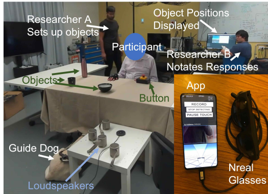
Figure 2. An example experimental setup is shown (reproduced from [23]). Note that twelve overhead cameras for the motion tracking are not visible.
