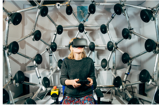
Figure 5. ARI: The loudspeaker array studio (LAS) consisting of 91 loudspeakers for listener-specific HRTF measurements and behavioral experiments requiring a direct comparison between the loudspeaker-based and binaural sound reproduction.
