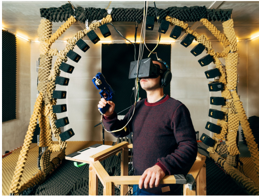
Figure 4. ARI: Yellow booth showing the sound-source localisation setup consisting of a VR goggles and a pointing device.
