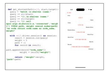
Fig. 5: Code and UI for shortest path identification.
