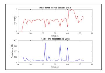
Fig. 4.Graph depicting Force and Resistance values generated from the force sensor in MATLAB.
