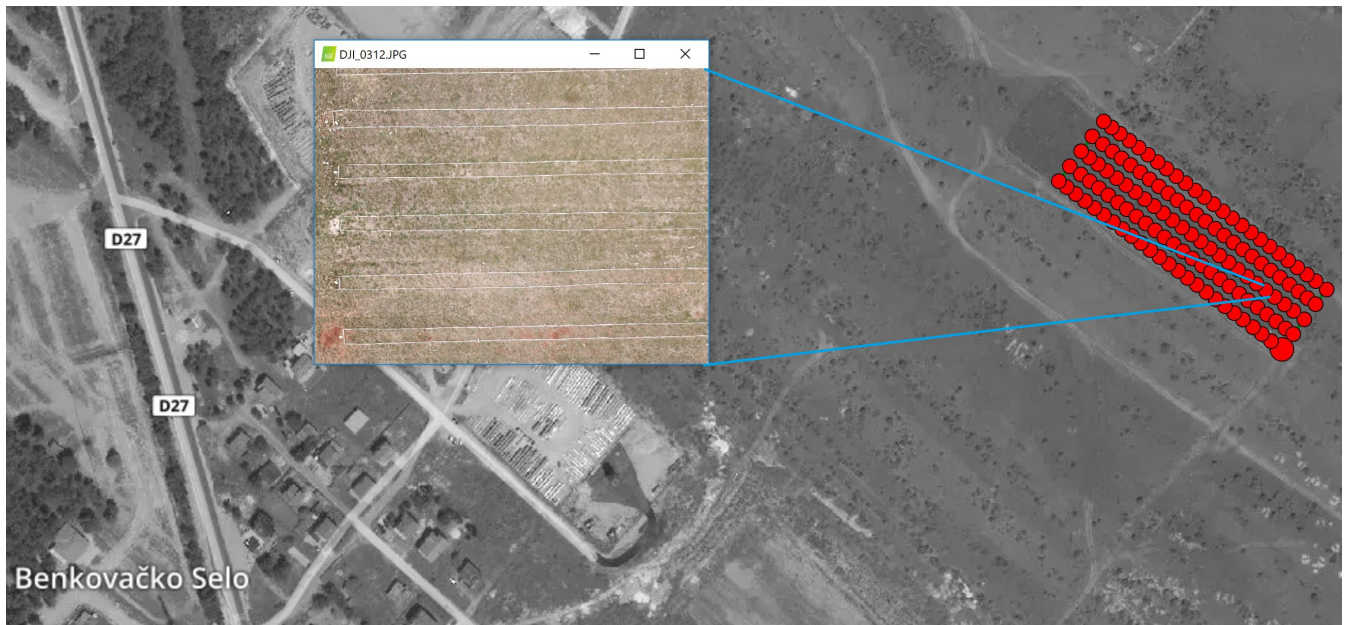
Fig. 8: Geo-mapping of 125 frames captured by the Multispectral Parrot SEQUOIA+ camera a larger terrain than the land fields starting from the biggest circle to the left and to the right using Pix4DMapper.
