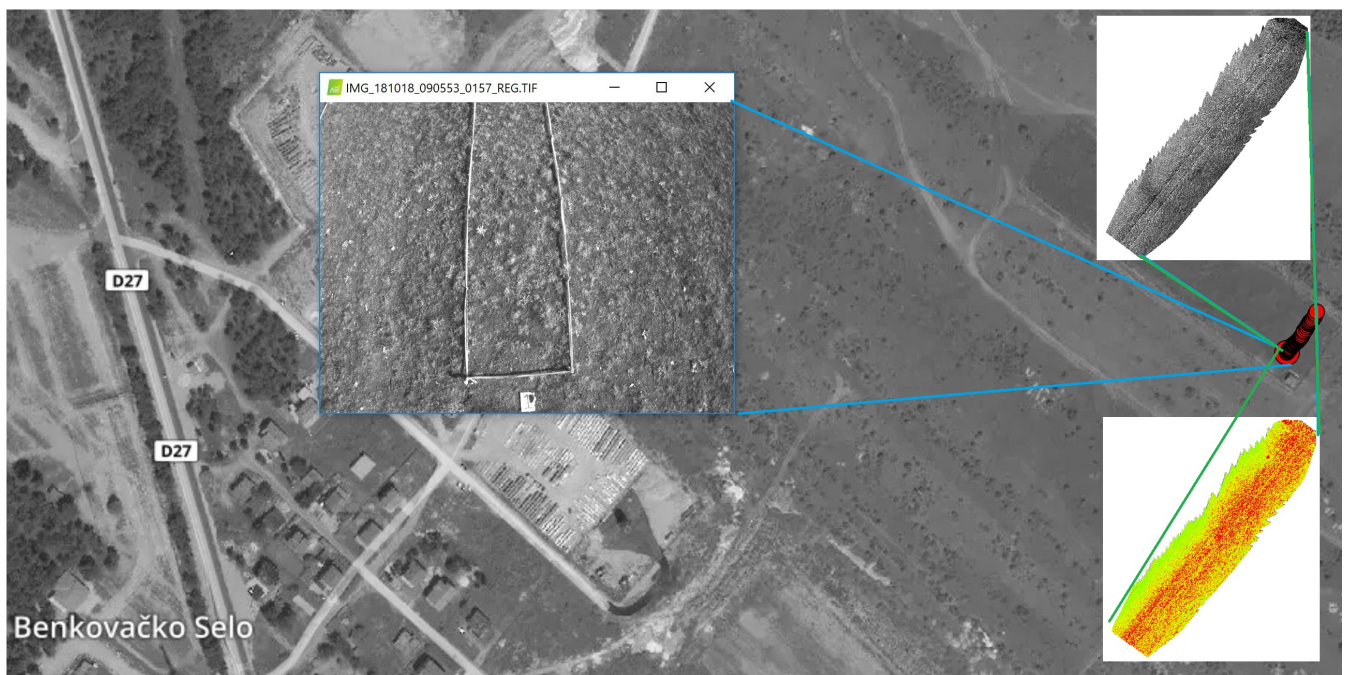
Fig. 9: Geo-mapping of 172 frames captured by the Multispectral Parrot SEQUOIA+ camera on the lane1 starting from the biggest red circle using Pix4DMapper.
