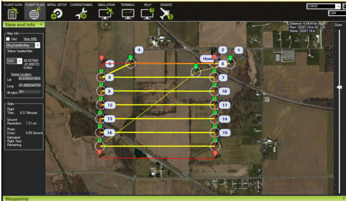
Fig. 2: The route specification interface of the UAV with respect to geospatial map for autonomous use of the UAV.
