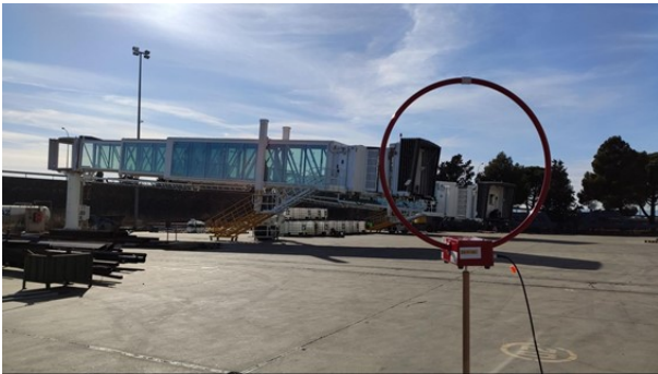
Fig. 7. Case study 2. Photo of the in situ setup for magnetic field emissions measurements from a passenger boarding bridge.
