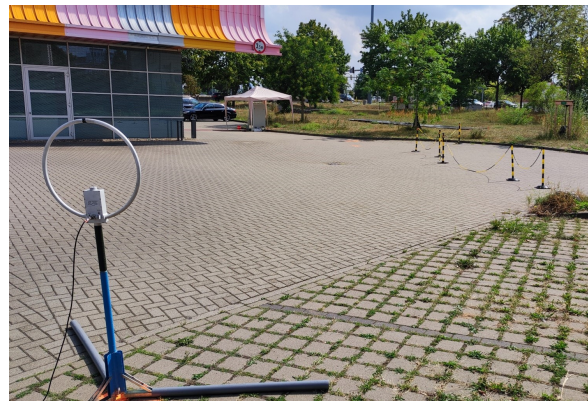
Fig. 4. Setup used for in situ magnetic field measurements for the PV system (Case study 1). Distance to the EUT is 30 m. Buildings may have an influence on the measurements, however this was out of the scope of this study.
