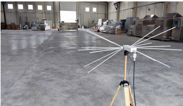
Fig. 11. Setup used for in situ radiated field emissions measurements from the pallet washing tunnel in an industrial warehouse (Case study 3).
