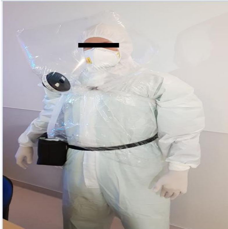
Figure 1: Single use low cost powered air-purifying respirator (PAPR) developed and used for airway procedures in the COVID-19 intensive care unit.
