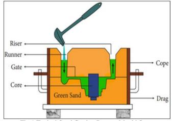
Fig 1 Typical Sand Casting Process Mould Setup
