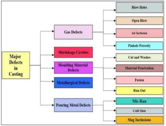
Fig 2 Basic Categories of Sand Casting Defects
