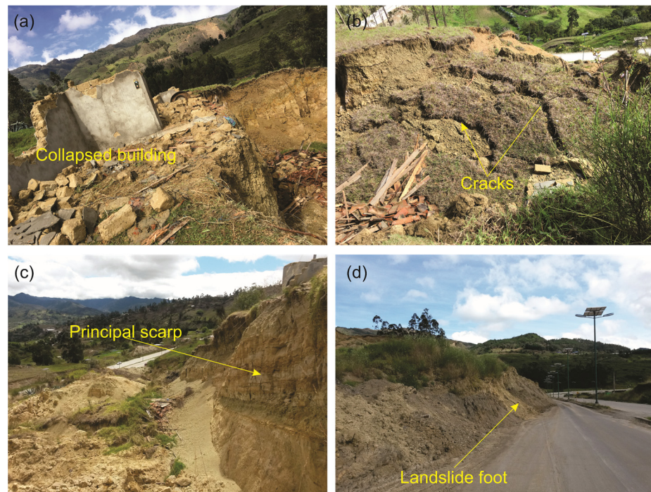
Figure 2. (a) Collapse of houses due to slope movement activity; (b) Presence of cracks in the slope body; (c) View of the main scarp on the southern flank of the slope; (d) Accumulation zone along the roadway.
