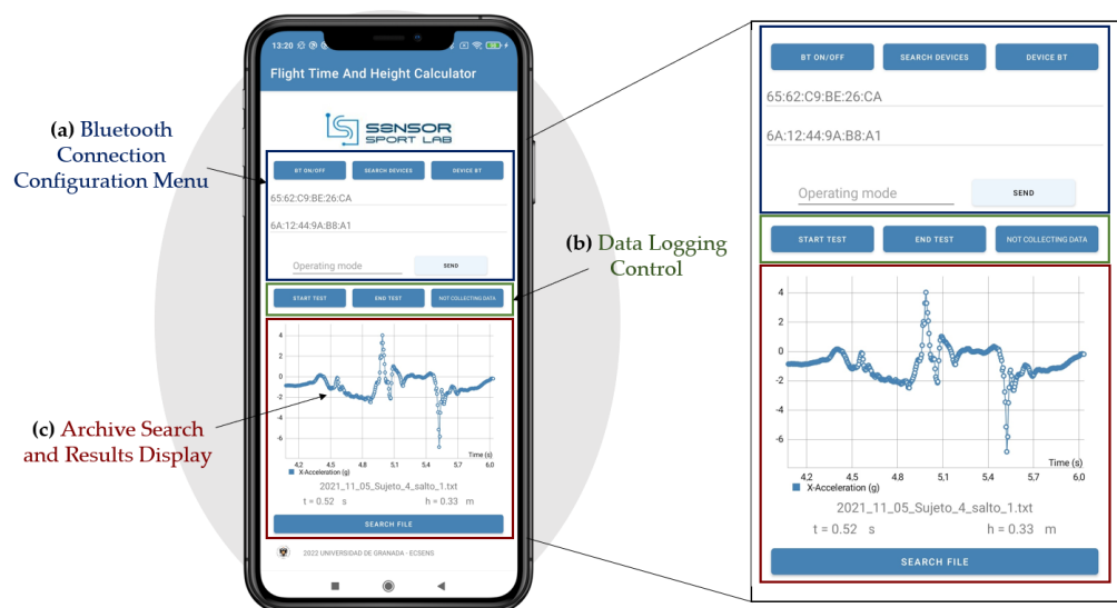
Figure 3. Overview of the custom smartphone application: (a) Bluetooth connection configuration menu; (b) Data logging control, used to initiate and terminate data acquisition and storage; (c) Archive search and results display.
