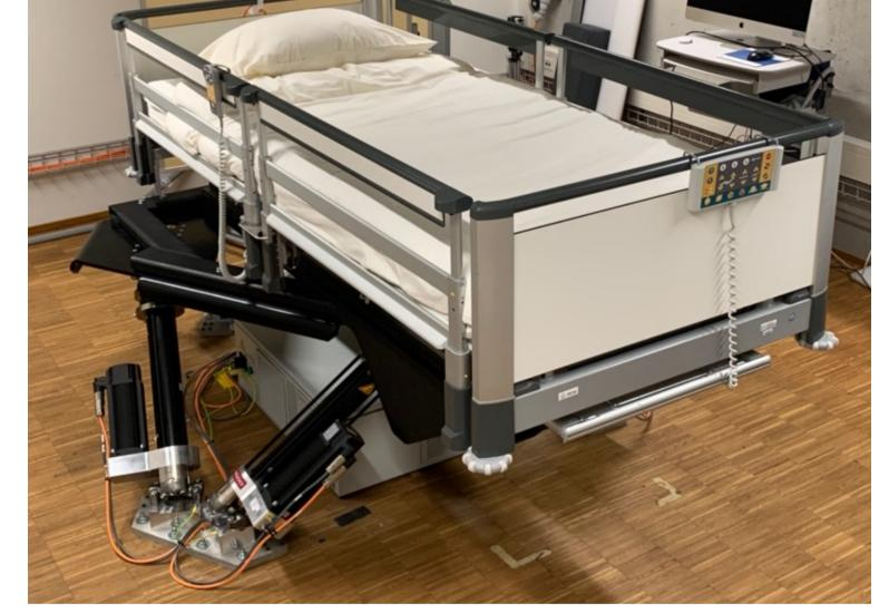
Cocktail of rotation (yaw, pitch, roll) at .25 Hz during sleep using a bed mounted on a 6 DoF motion platform.
