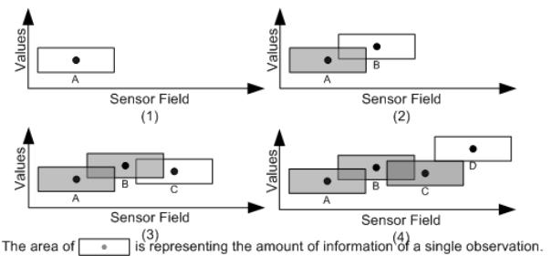
Figure 3. The vector quantization system of observations and the relative information gain process of an observation.
