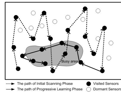
Figure 1. The working process of proposed sensor visiting strategy.
