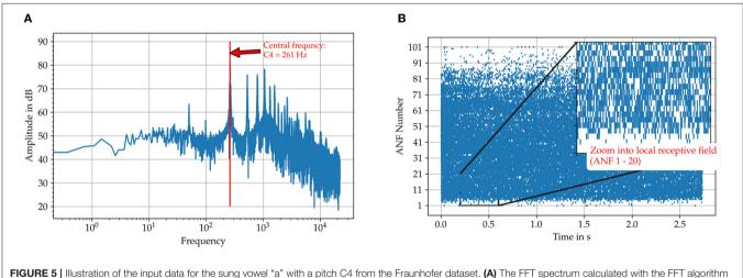
FIGURE 5 | Illustration of the input data for the sung vowel "a" with a pitch C4 from the Fraunhofer dataset. (A) The FFT spectrum calculated with the FFT algorithm included in the Python package SciPy. (B) The spike trains on the auditory nerve fibers originating from the SAM model. Those are used as direct input to the octopus' neuron model.
