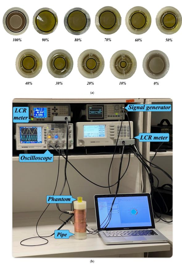
Figure 6. (a) Different void fractions generated by the phantoms. (b) Experimental setup.
