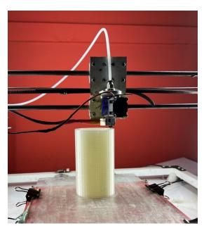
Figure 4. 3D printing of a pipe with a transparent PLA filament.
