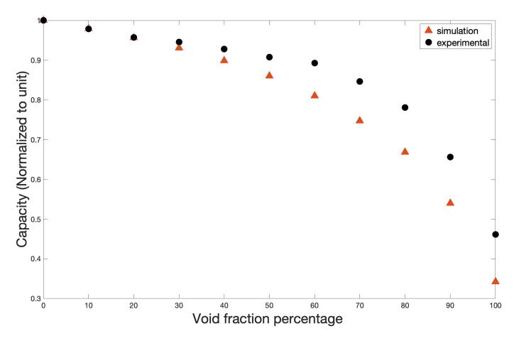
Figure 11. Comparison of the experimental data and the simulated data in a two-phase annular flow.
