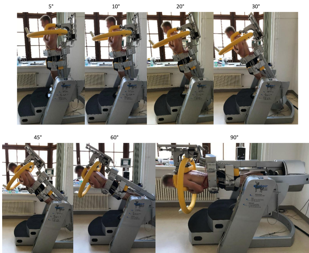
Figure 1. Applied tilt angles for the determination of the EMG amplitude–force relationship. Note that the upper body is always aligned along the body axis and the arms are held crossed in front of the chest.
