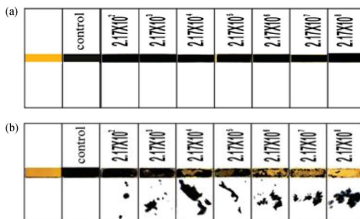
Fig. 1. a) Colorimetric Listeria monocytogenes protease sensor probe using D-amino acid covalently bound to a magnetic nanobead; a) before adding the sample to the specific Listeria monocytogenes protease substrate; b) after adding different concentrations of Listeria monocytogenes protease solutions. (For interpretation of the references to color in this figure legend, the reader is referred to the web version of this article.)
