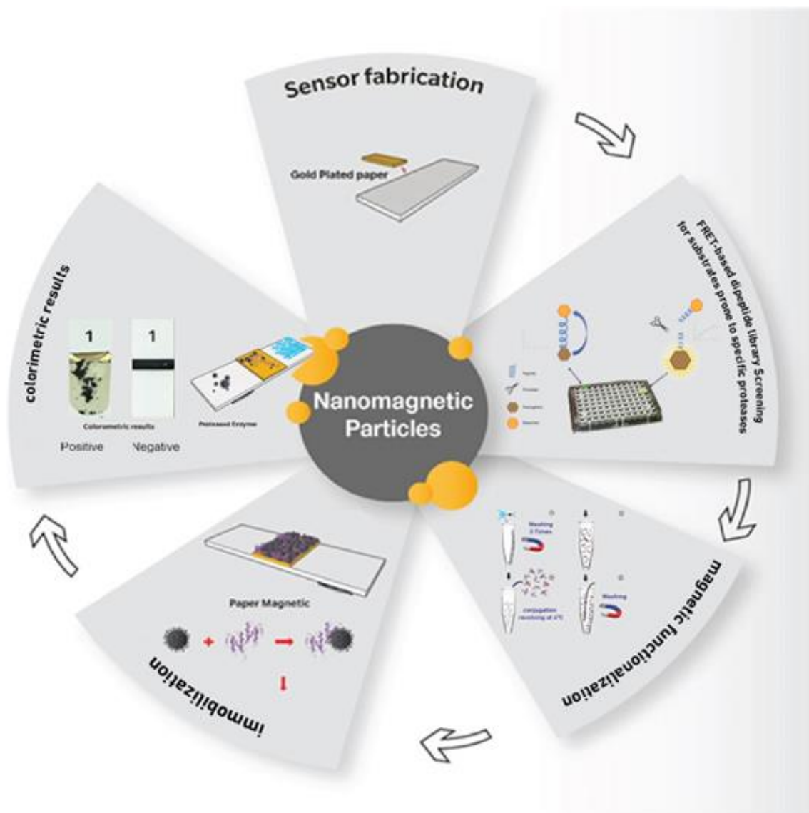
Figure 1.3: Schematic diagram representing the steps involved in this project, including sensor fabrication, dipeptide library screening, functionalization of the nanomagnetic peptide sequence with nanomagnetic particles to form a complex, immobilization of the complex on the sensor platform, application of the enzyme, and colorimetric test results.
