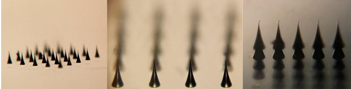
Figure 10: Conical Fiber Tips Batch – printed by 3D laser lithography.
