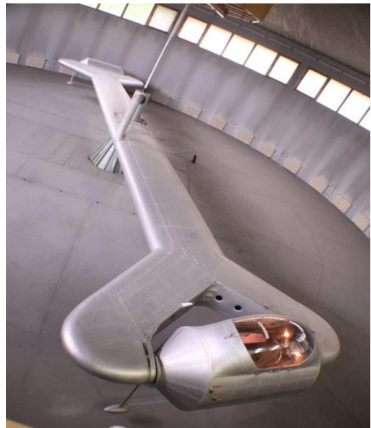
Figure 1. Human centrifuge motion simulator installed at Aero Medical Institute in Belgrade
