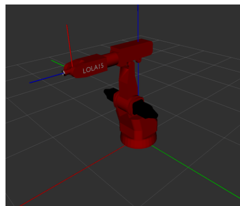
Figure 4. LIRL15 model at the initial configuration in RViz.
