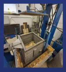
LIWEMAT investigates deformation characteristics of two types of lightweight materials - foamed glass aggregates and expanded clay aggregates to be used in infrastructure projects.
