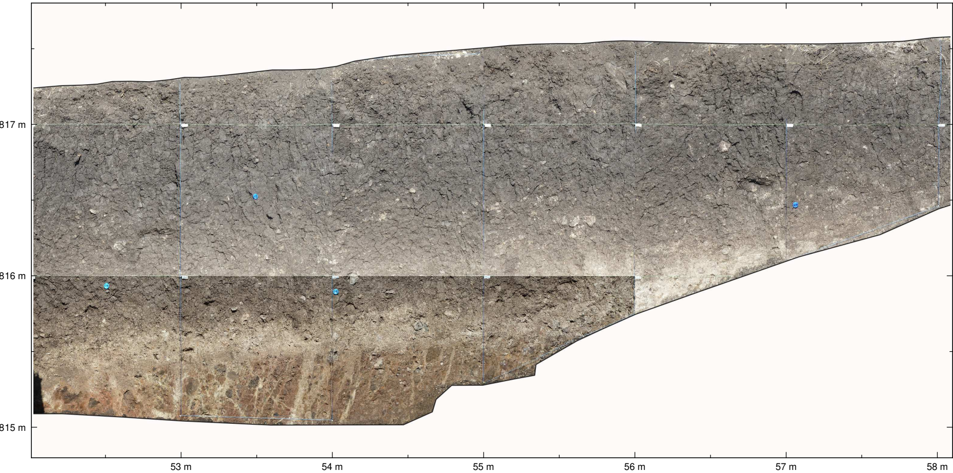
Figure SI.3: Photomosaic of the NW trench wall, f2 fault damage zone
