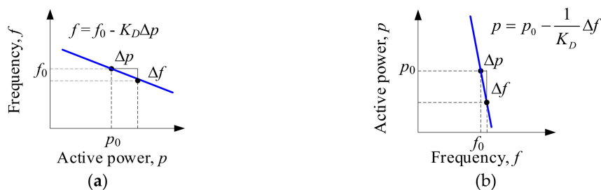
Figure 2. Comparison of the operational characteristics according to the droop action: (a) synchronous generator governors and (b) virtual inertia (VI) systems.
