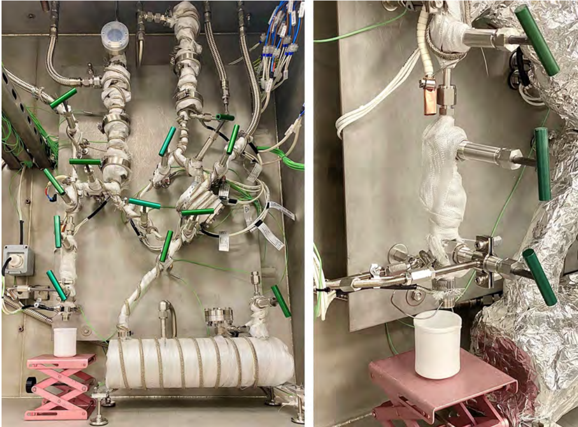
Fig. 8.11. [Left] Assembled liquid lithium system of the LYDER experiment wrapped with fiberglass tape and ten heating wires. [Right] Removable sample holder without thermal insulation surrounded by a heating cable and fiberglass tape. It is connected to the lithium system by a VCR fitting heated by a small cartridge heater.
