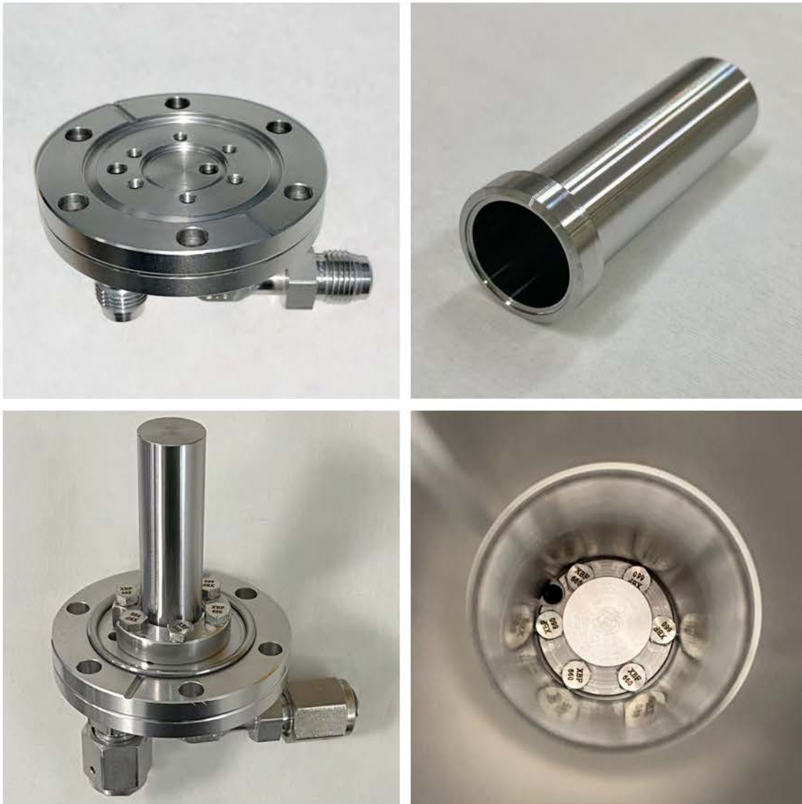
Fig. 8.14. [Top left]: Modified DN40CF blind flange used as the base for the deuterium injection system. It has a custom DN16CF knife-edge in the center surrounded by six blind M4 threaded holes. The liquid lithium enters through a drilled hole between the two knife-edges on the left, and the ^2\text{H}_2 gas enters the tube through the hole inside the DN16CF knife-edge. [Top right] Fabricated closed \alpha -iron tube acting as a deuterium permeation membrane with a DN16CF knife-edge at the open end. The tube is attached to the center flange of the base plate by a conventional DN16CF flange ring using a DN16CF \alpha -iron Helicoflex ® gasket. [bottom left] Assembled deuterium injection system with a DN40CF \alpha -iron Helicoflex ® gasket sitting on the outer knife edge. [bottom right] Top view into the right tank showing the deuterium membrane from above. The picture shows the hole through which the liquid lithium enters.
