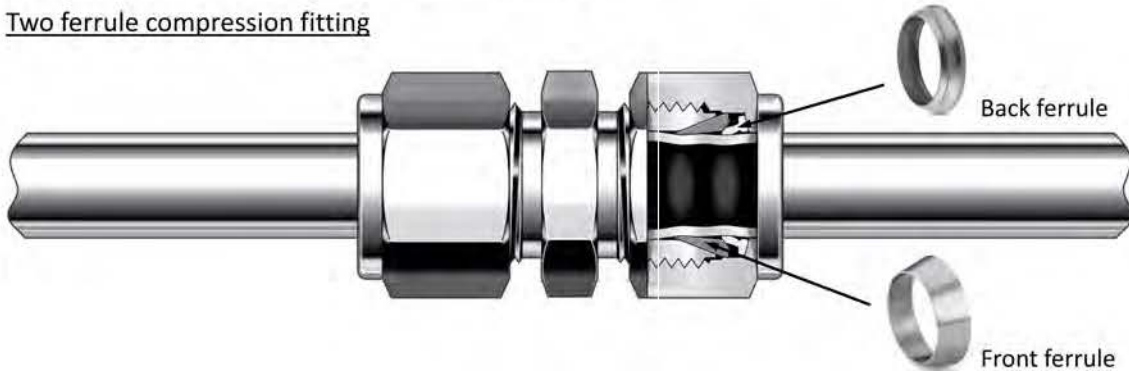
Fig. 3.3. Section cut through a typical commercially available [top] metal gasket face seal (VCR®) fitting [200] and a [bottom] two ferrule compression fitting [202] made entirely of 316 stainless steel.
