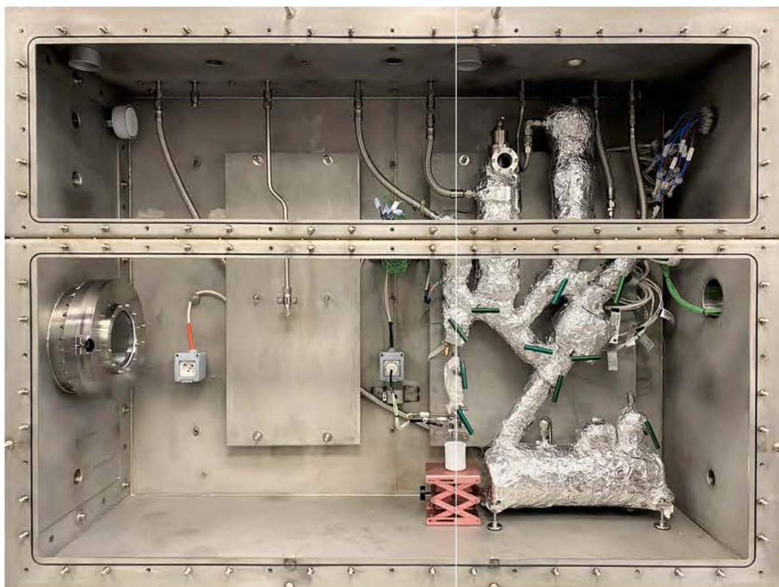
Fig. 8.4. Interior glove box components of the LYDER experiment involving a branch for TDS experiments on the left and the lithium system on the right.
