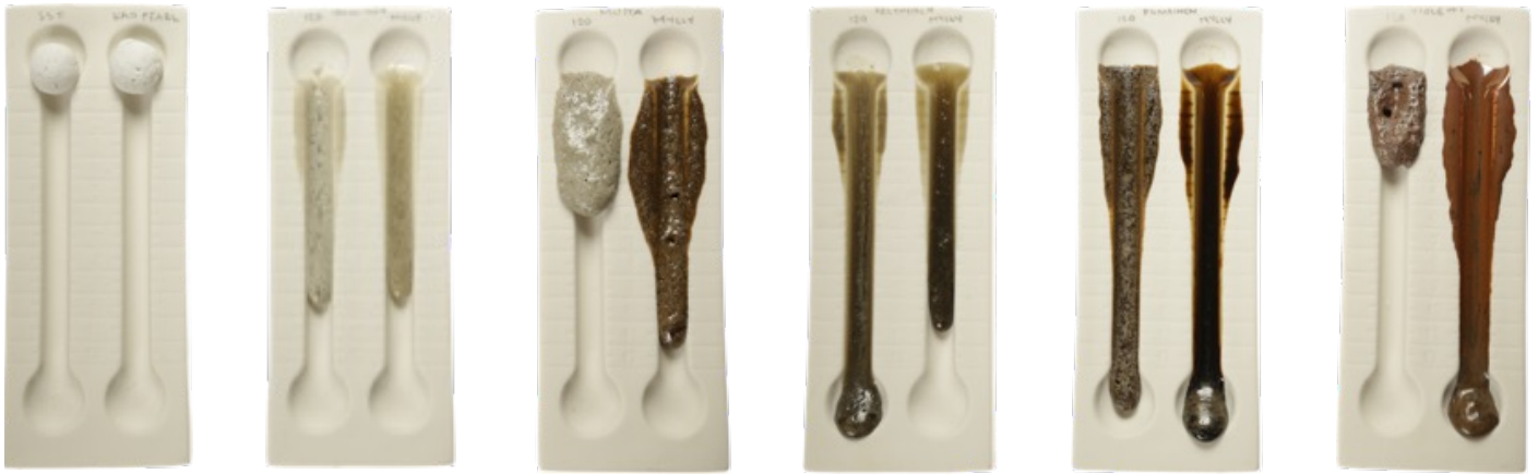
Picture 3. Viscosity tests. 1st commercial Super Standard porcelain and KaoPearl. After that Pihlajavaara white, black, yellow, red, and purple. Left side is \leq 120 mesh and right side milled.
