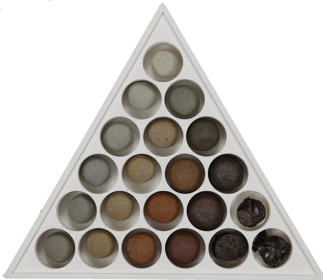
Image 7. Triangle test with Pihlajavaara white and black and Rannikonmäki earthenware, fired to 1250°C in electric kiln.
