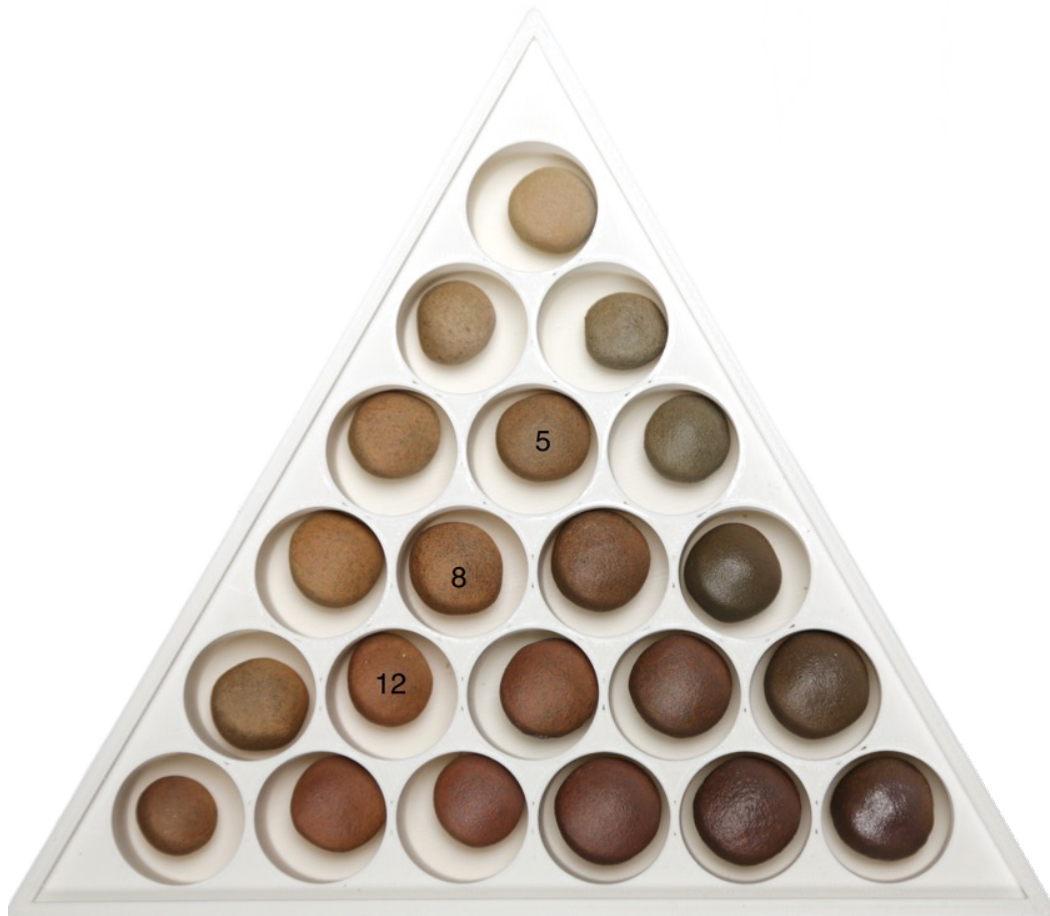
Image 6. Triangle test 2 for Pihlajavaara white, black and Saarijärvi clay. Gasfired in reduction 1235°C.
