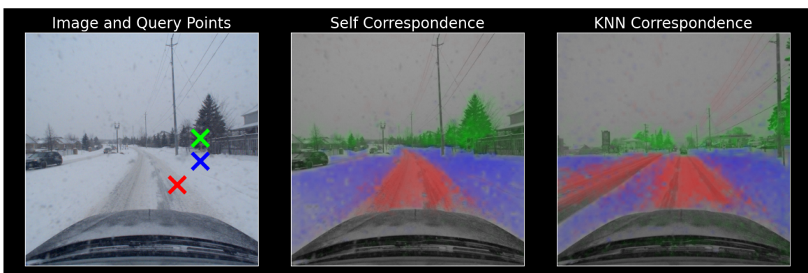
Figure 3.9: Feature correspondence between DINO features in winter driving scenario. Each heatmap color represents correspondence with the sample location of the same color. The plotting tool is adapted from [32].
