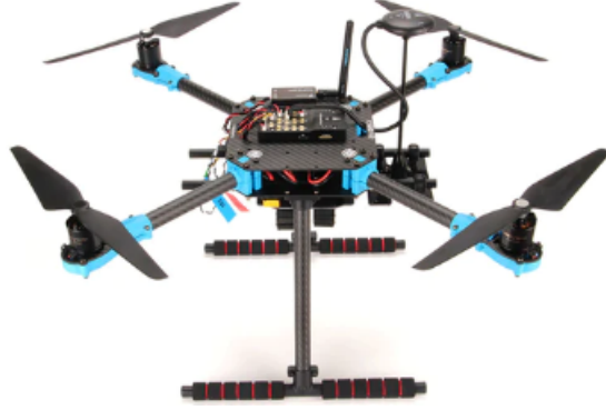
Figure 6: The X500 UAV setup with the PX4 flight controller
