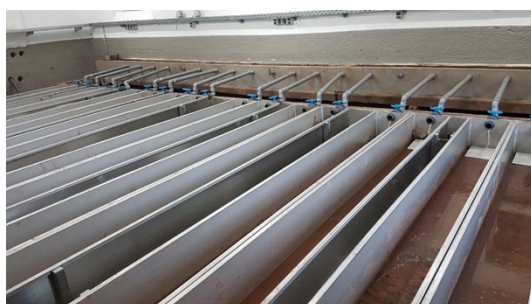
Figure 3. Artificial stream channels used in particle fate experiments 1 (indoor metal flumes)
