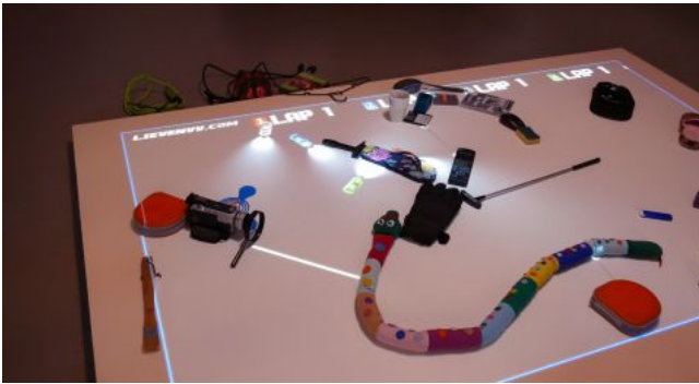
Figure 3: Photograph of Room Racers, a spatial augmented reality racing hybrid board game that involves AI as part of the racing track generation.
