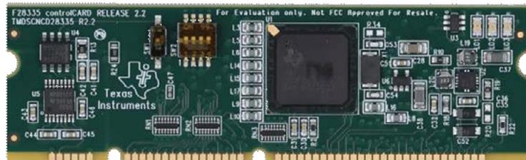
**Figura 4:** Controlador TMS320F28335 de Texas Instruments.
