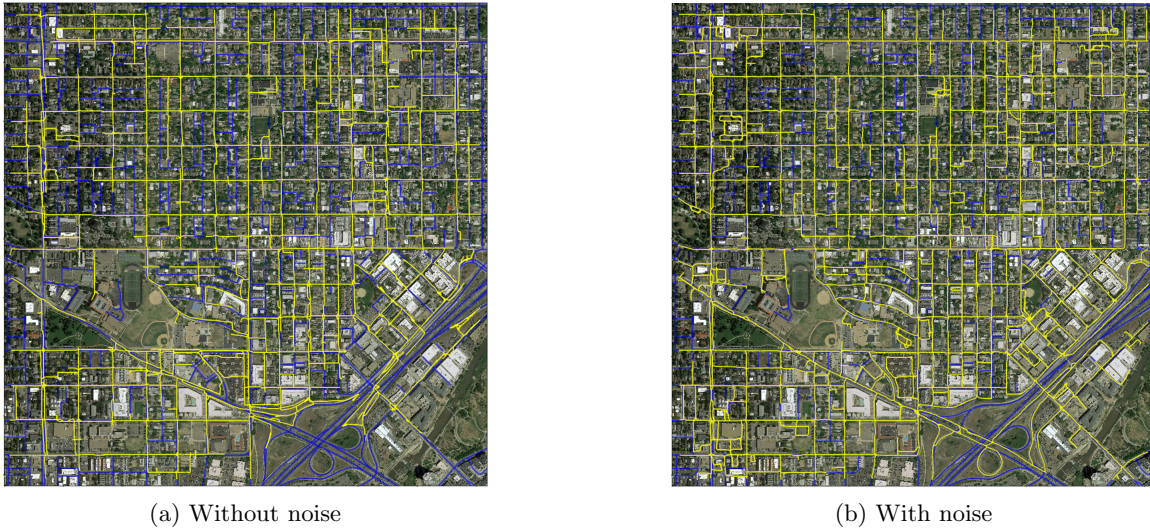
Figure 4.5: Graphs created with the proposed method if trained (a) without noise, or (b) with noise. The ground truth is marked with blue lines, while outlined in yellow are the roads detected by the network and graph exploration algorithm.
