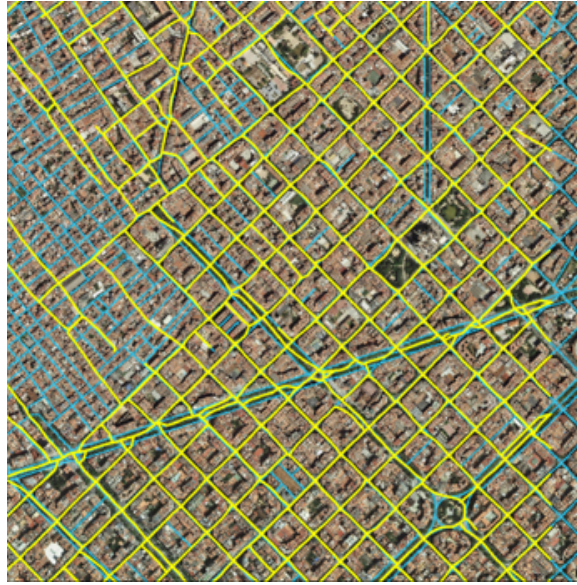
Figure 2.9: Representation of all roads visible in Barcelona from a Satellite image. Outlined in yellow are all the roads that a model trained to extract roads via graphs has been able to detect. The lack of yellow overlapping the blue ones indicates that the network has failed to detect valid roads.
