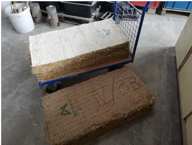
Fig. 1. Straw quilt specimens with 50 × 100 cm production sizes (photo: Rebeka Ábrahám-Horváth)
