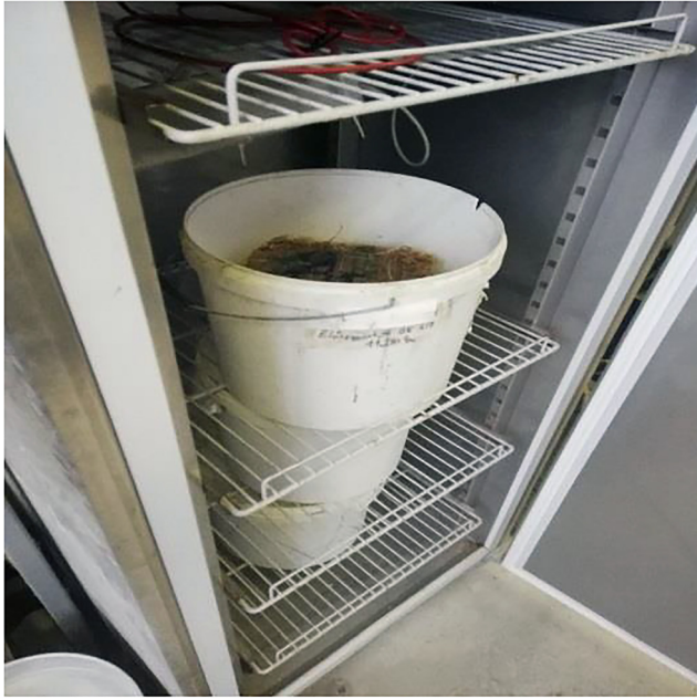
Fig. 3. Straw quilt samples in the freeze-thaw chamber (photo: Rebeka Ábrahám-Horváth)
