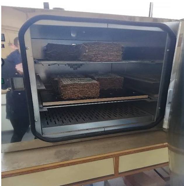
Fig. 2. Straw quilt samples in the drying oven (photo: Rebeka Ábrahám-Horváth)
