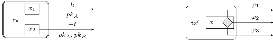
Fig. 1. (Left) \text{tx} is published on the blockchain. The output of value x_1 can be spent by a transaction containing a preimage of h and signed w.r.t. pk_A . The output of value x_2 can be spent by a transaction signed w.r.t. pk_A and pk_B but only if at least t rounds passed since \text{tx} was accepted by the blockchain. (Right) \text{tx}' is not published yet. Its only output can be spent by a transaction whose witness satisfies \varphi_1 \vee \varphi_2 \vee \varphi_3 .
