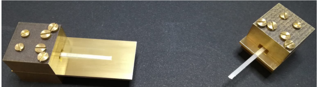
(a) DIL rod antennas. Left: as discussed in Section 5.1.1, right: with short ground.
