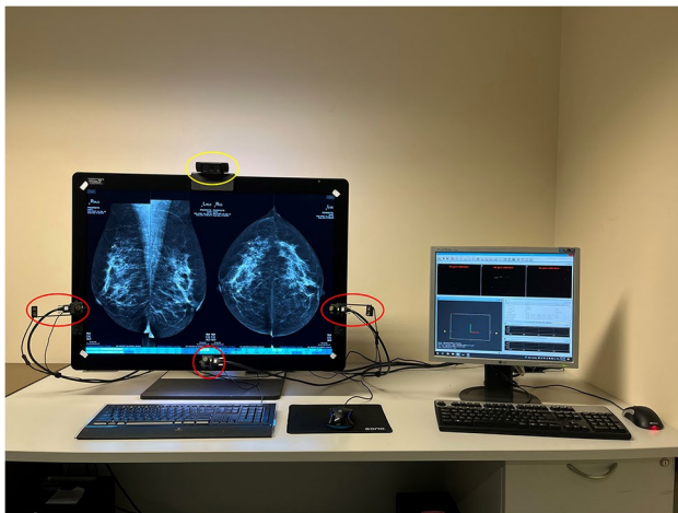
Fig. 1 Experimental setup. Eye tracking cameras (red circles) and a scene camera (yellow circle) positioned on a participant workstation. The monitor to the right was used for eye tracking calibration and monitoring. This was not visible to the participant during the experiment. During the experiment, the lights were dimmed
