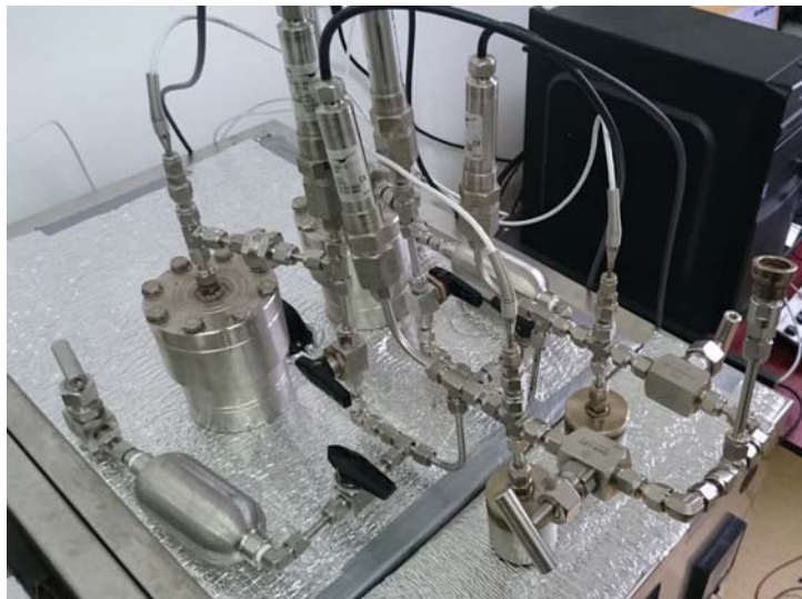
Figure 3. High precision manometric sorption setup from the Mining and Geology Faculty of the Silesian University of Technology
