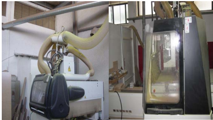
Figure 1. Model for encapsulating dust generating equipment
