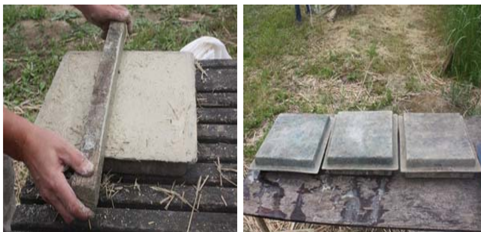
Figure 3. Pilot panels – Miscanthus Giganteus "bio-concrete"
