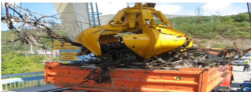
Figure 6. The floating debris collected by the grapples (the example from 'Bajina Basta hydropower plant')
