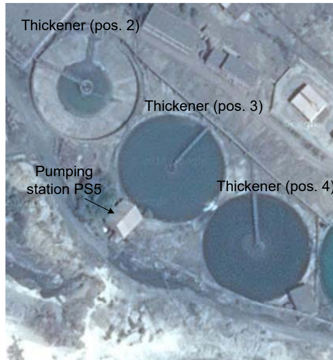
Figure 1. Thickeners for final tailings (taken from maps.google.com)
