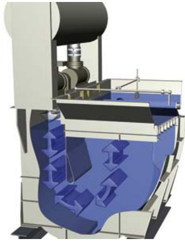
Figure 1. Principle of operation of ALLMINERAL pulse jig [6]
