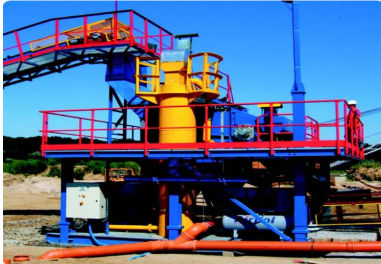
Figure 5. Pulse classifier developed by ITG KOMAG [7]
