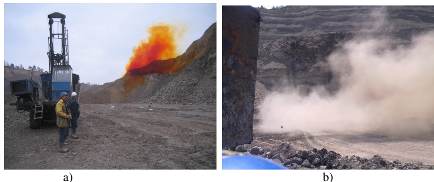
Figure 3. The post-detonation fumes a) non-ideal detonation b) ideal detonation
