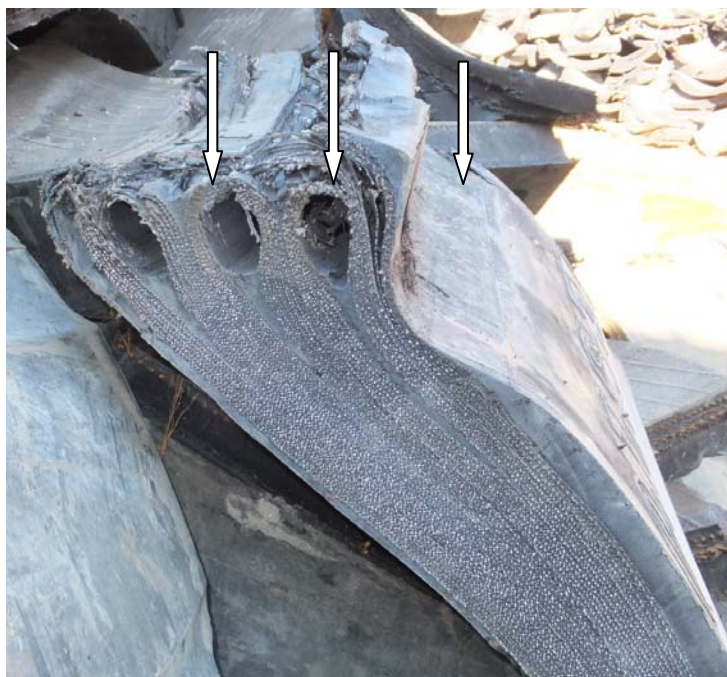
Figure 2. A cut through tire presenting the location of the steel wire rims (removed) and the cuts in the tire toe (arrow marked)
