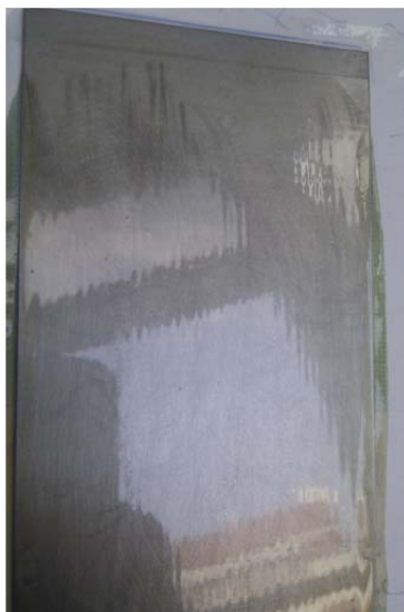
Figure 2. Dry films of the AR-TMP on metal plate
