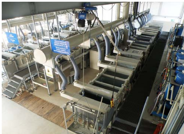
Figure 1. Drive electroplating and chemical protection in „ORAO“ a.d. Bijeljina (July 2012 image N.Bratić)
