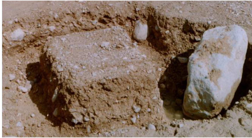
Figure 1. Sample for direct shear test and test body block [1].
