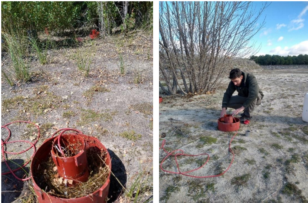
Figure 73. Infiltration tests inside a MAR infiltration ponds (EL Carracillo and Santiuste) to study the effect of vegetation on seepage rates.
