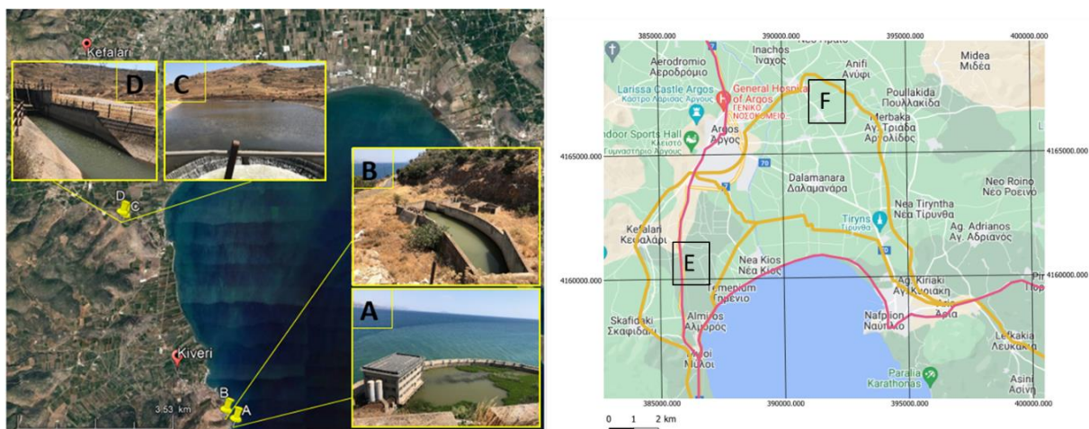
Figure 49. The infrastructure system of water management in the South part of the study area consisting of A) the Anavalos dam, where fresh water is collected and transported to the north through B) the Anavalos canal, mainly used for irrigation purposes. C) Is a buffer lake in Lerni, which is used as part of the transportation system of fresh water from Lerni Lake to the Argolis field through D) the canal network. On the right map E). The water pipes system is shown in red, and F) the irrigation pipes system (Anavalos and Nea Kios canals) is shown in yellow, respectively.
