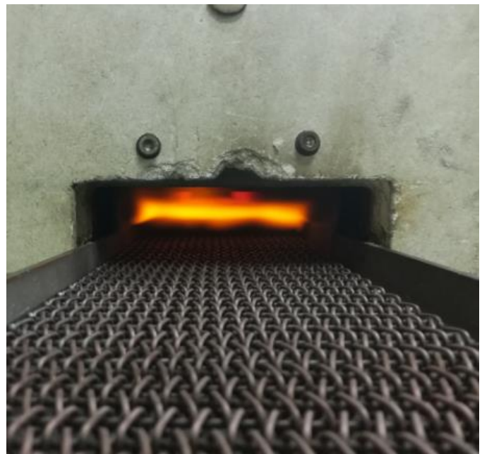
Figure 1. Appearance protective atmosphere at the entrance to the furnace
