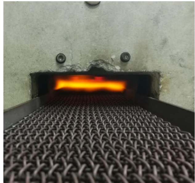
Fig. 2 Appearance protective atmosphere at the entrance to the furnace
