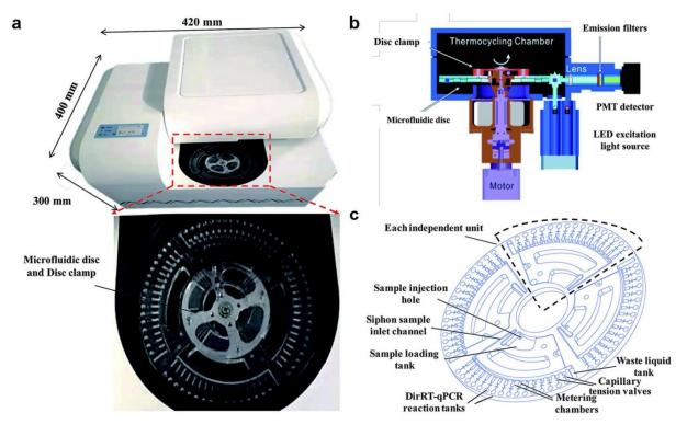
**Figure 5.** (a) A photograph showcasing a compact and portable centrifugal microfluidic device; (b) a schematic diagram illustrating the different components of the microfluidic device; and (c) a schematic illustration highlighting the structure and functional regions of the centrifugal microfluidic chip (adapted with permission from Ref. [83], copyright 2020 Royal Society of Chemistry).
