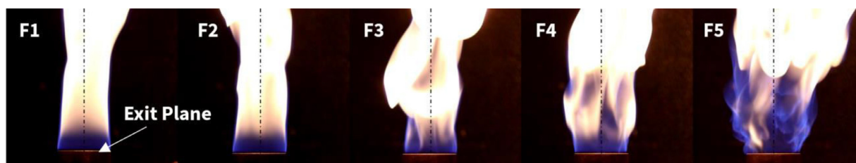
Fig. 5. Instantaneous DSLR images showing the onset of soot formation and oxidation near the burner exit plane for all flames with increasing fuel-turbulence.
