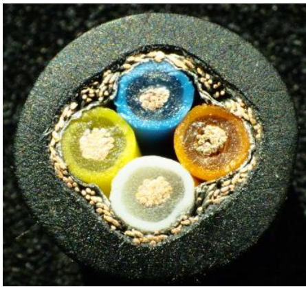
Fig. 3. Cross-section of a typical 4-wire RailCat 5e twisted-quad cable with nineteen conductor strands
