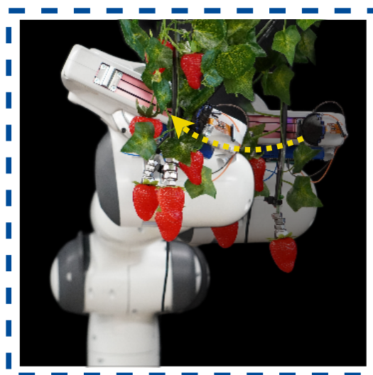
Figure 7. Physical manipulation of harvesting environments using tactile sensation: strawberry cluster manipulation using visual tactile sensor.
