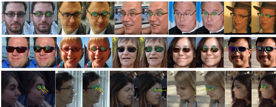
Figure 5.13: Results from applying our model on faces with glasses (1st row), sunglasses (2nd row) and faces in near-profile pose (3rd row). While normal glasses do not pose a significant challenge, sunglasses and profile poses are more difficult to handle.
