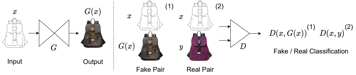
Figure 2.8: A diagram of the pix2pix model and data flow during training. Pairs of images of the same scene/object but in two different domains are used to train the Generator. The Discriminator is trained with pairs of images where the target domain image is either a real or a generated one. Images are taken from the original paper [17].
