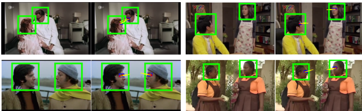
Figure 5.8: Visualisation results of our multi-face gaze estimation on the AVA-LAEO dataset. Our single pass gaze estimation method, trained with a large collection of “in-the-wild” and controlled images, is useful for improving detection accuracy of the LAEO task in real conditions.
