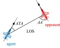
Fig. 1. ATA, AA, and LOS geometric representation.
