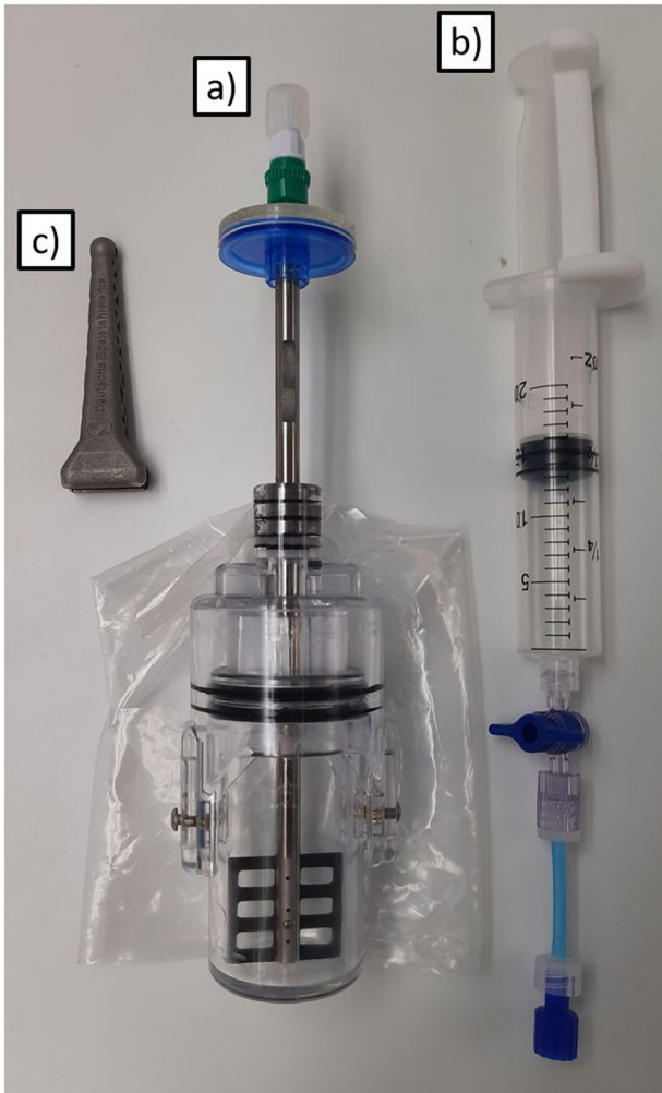
Fig. 1 Items of a MASON Kit. a MASON Concrete Mixer, b syringe and c crank.
