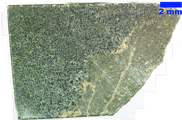
Figure 1. Reflected light image of ID 500 acquired with Keyence Digital Light Microscope VHX-500F. The sample consists mainly of metallic iron (dark-gray) at the left-hand site and silicate material on the right-hand site.
